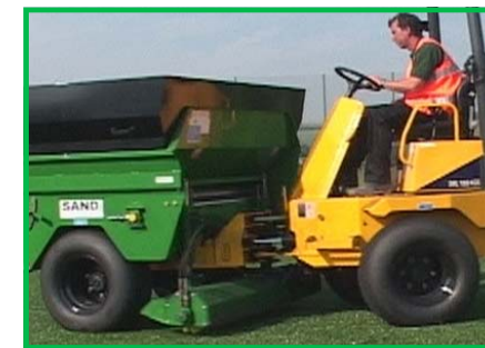
Articulated steering helps prevent carpet movement and rucking
