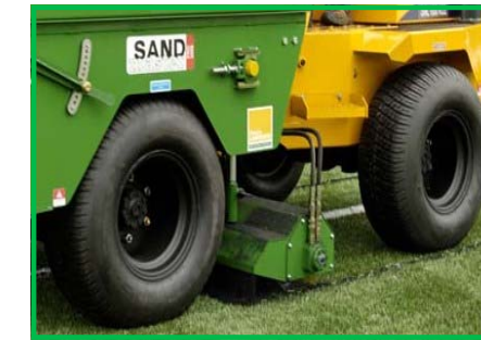
4 large tyres give better weight distribution and lower ground pressures
