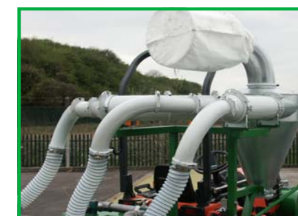
Dust collection system
